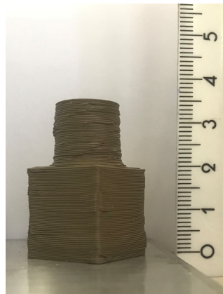
Figure 2. As built part before milling.
